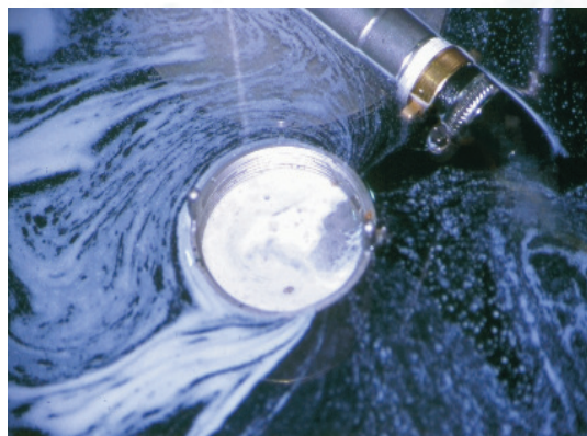
The oil films follow the hydraulic gradient and can be separated.
